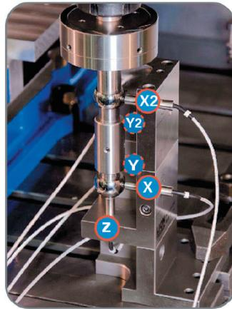
Note: Two of the sensors (Y Y2) are located behind the dual-masterball target.
