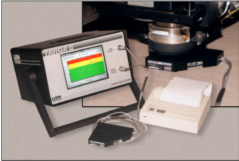
Figure 1. Measurement of high-speed spindle runout is now possible using a noncontact transducer and electronics.
