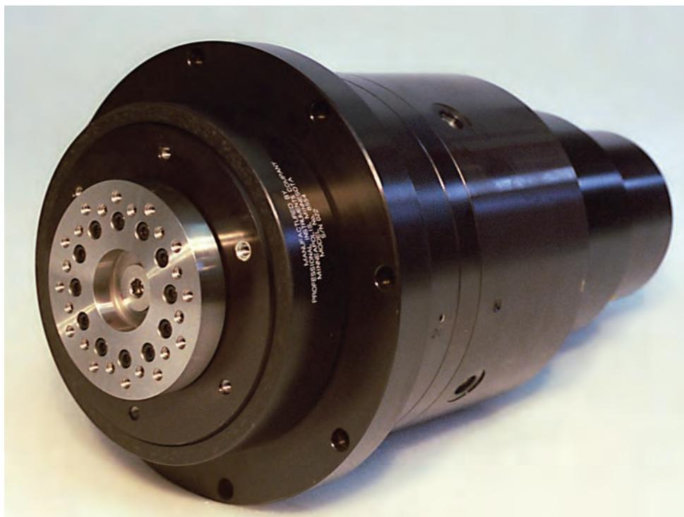
**Figure 5.13** The PI 5.5 ISO is designed for maximum accuracy in a compact package. Its captured thrust between large radial bearings provides high stiffness in a spindle that can be operated at high speeds.
