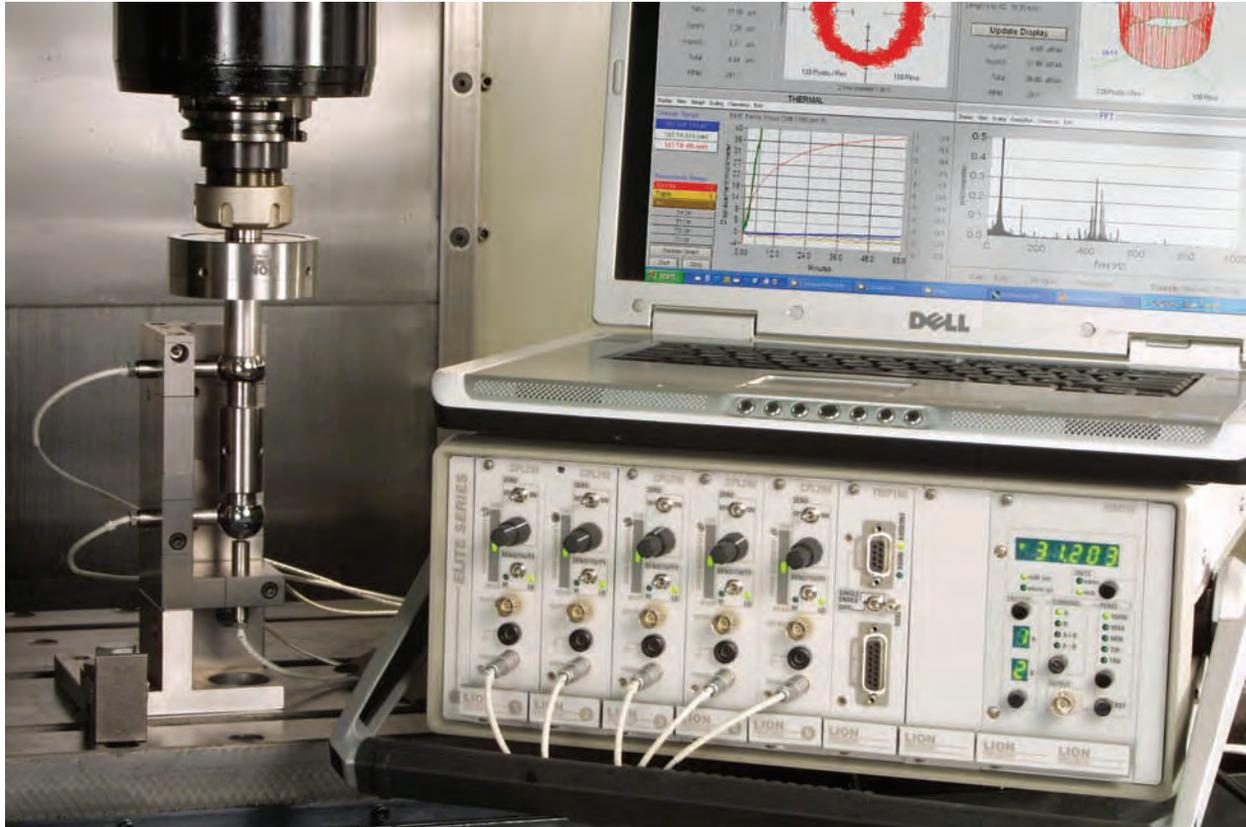
**Figure 5.11** CNC vertical machining center with variable speed, AC motor and angular contact, ball bearing spindle.. The probes are configured for measuring motions capturing all five degrees of freedom. The probes are located in the place of the tool and will measure the combination of spindle error, structural error, and the effects of any disturbances to the machine.
