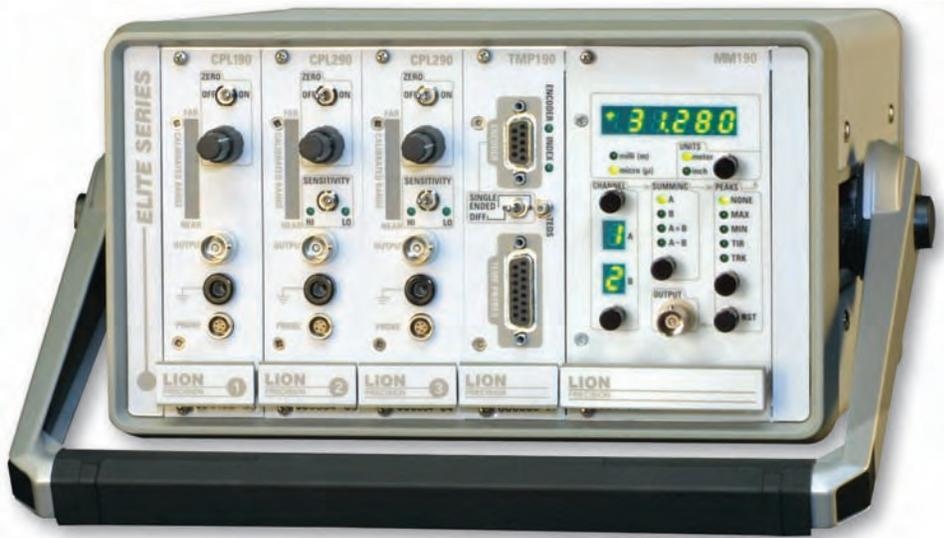
**Figure 3.7** Lion Precision 3-channel CPL290 capacitive probe driver with MM190 LED display. The output from each channel is a  $\pm 10$  V analog signal that can be electronically zeroed at an arbitrary gap distance. This particular modular system is also configured for multi-channel temperature measurement and encoder input using the TMP190 module.
