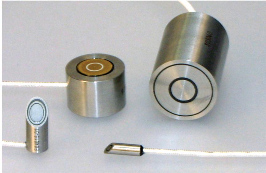
**Figure 3.6** Custom-made capacitive probes from Lion Precision for special applications. These probes are shielded, temperature compensated, and factory calibrated for linear outputs over their measurement range. A comprehensive line of standardized probes is also available from Lion.
