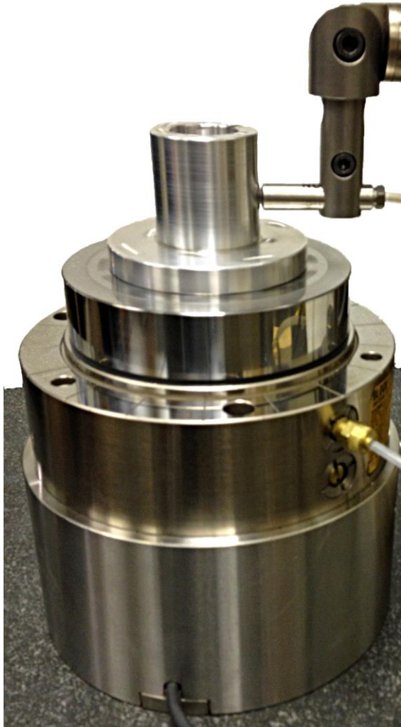
FIGURE 5. Measurement of the out-of-roundness of an aluminum target using a Lion Precision C1-C capacitive sensor.
