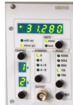
*When using capacitive sensors, TIR can be displayed with the MM190 Meter Module.*
