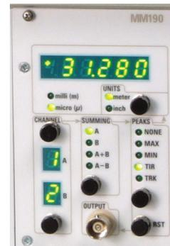
“Total Vibration” can be displayed with the TIR function on the MM190 Meter Module.
