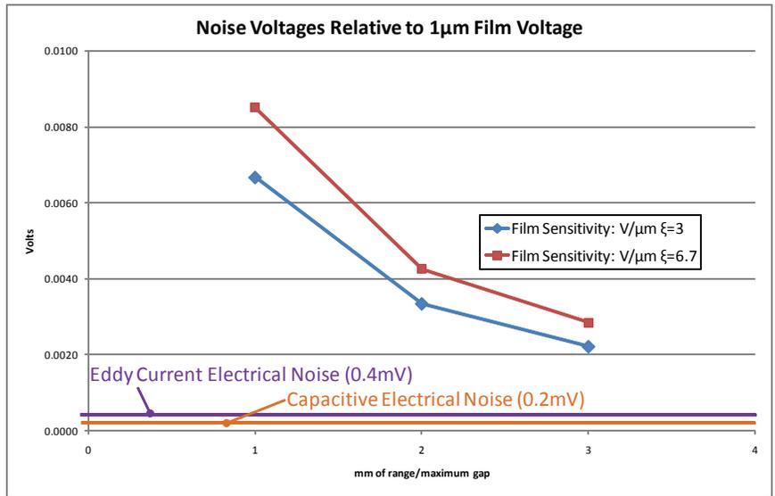
Magnitudes of film sensitivity and error sources are generalized approximations. Specific values will depend on final system configuration.
