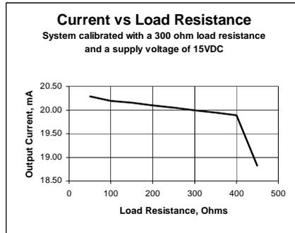
It is possible to adjust the current output to achieve 4-20mA if required. Contact Lion Precision for details.
